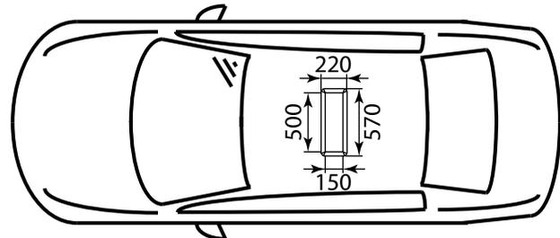
Fig. 1: Exemplary location of the chassis antenna cavity on a car roof. All dimensions in millimeter.
