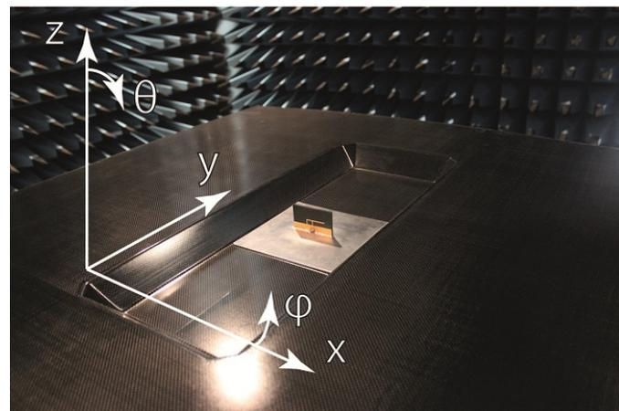
Fig. 3: Inverted-F antenna for 2 GHz inside the CFRP antenna cavity prototype.
