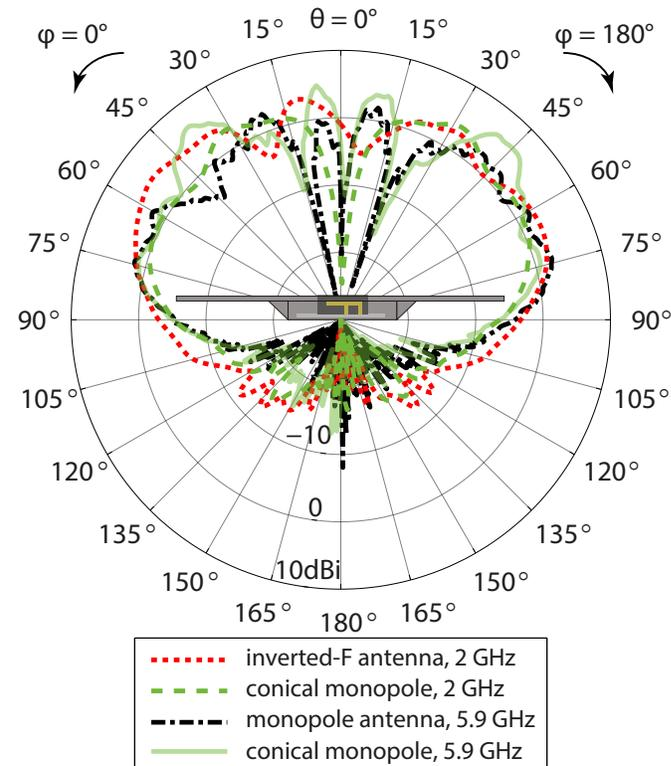
Fig. 5: Measured gain patterns of the IFA at 2 GHz and the monopole antenna at 5.9 GHz inside the cavity, vertical cut for  $\varphi = 0^\circ$ .
