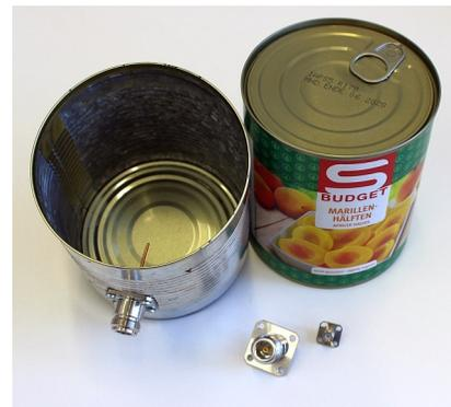
Fig. 5. A kit with canned food and coaxial flanges alongside a finished cantenna.
